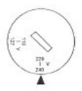
Set the selector so that arrow points to power voltage of your area. (Figure shows arrow pointing to 110 - 127 volts.)
