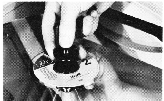
FIGURE 8 PRESS CENTER SHAFT DOWN
