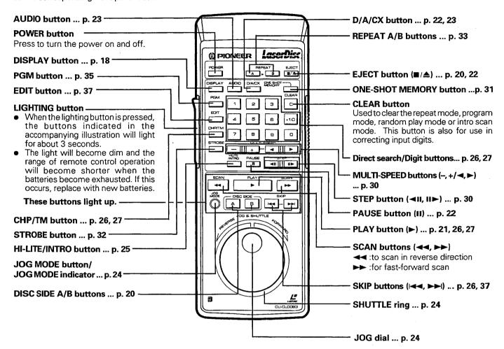
When operating the remote control unit, point the unit's infrared signal transmitter at the remote control receiver on the front panel of the player. The remote control unit can be used within a range of about 7 meters (23 feet) from the remote sensor, and within angles of up to about 30 degrees.
