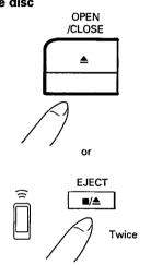
After removing the disc from the disc table, press  $\triangle$  or PLAY  $\blacktriangleright$  to close the table.
