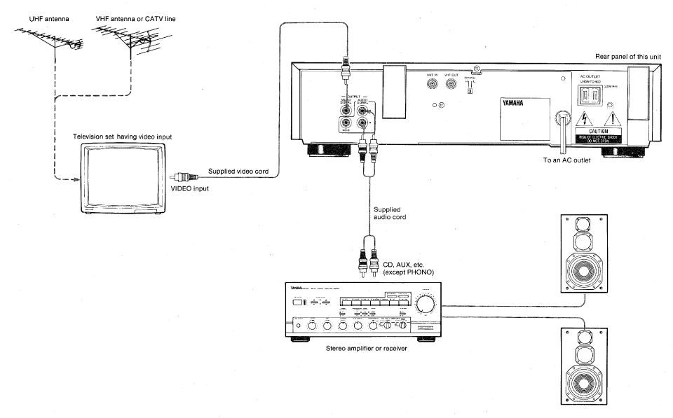
With a stereo amplifier or receiver having audio and video inputs and television set having video input
