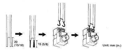
2. Plug the antenna adapter into the ANT IN terminal of this unit firmly.
