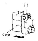
6. Plug the 75-ohm/300-ohm antenna adapter into the ANT IN terminal of this unit.
