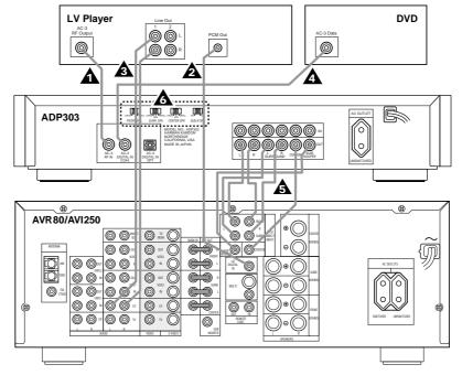
Use this setup for connection to an AVR80, AVI250 or other compatible products equipped with 6 Channel Direct inputs.
