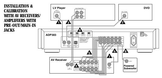
Although AV receivers that have both preout/main-in jacks for all five surround channels as well as a subwoofer output were not designed for Dolby Digital applications, you may use them with the ADP303 by using the following steps:
