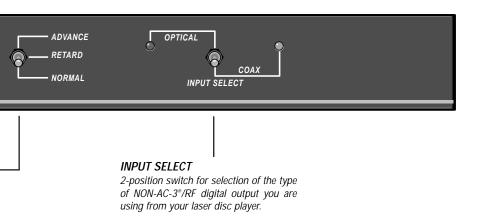
Connections between the SDP-RFD AC-3\*/RF Demodulator and associated equipment should be made with all units UNPLUGGED!
