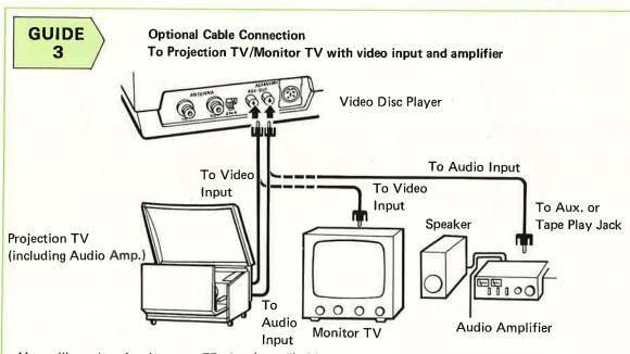
You will need a pin plug type 75 ohm (round) video cable and an audio cable. Neither of these cables is supplied with your Video Disc Player.
