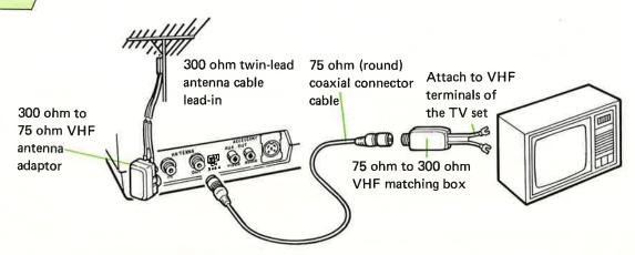
You will need the 300 ohm to 75 ohm VHF antenna adaptor (Accessory No. 3), the 75 ohm (round) connector cable (Accessory No. 2), and the 75 ohm to 300 ohm VHF matching box (Accessory No. 4), which are supplied with your Player.
