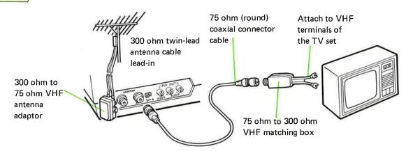
You will need the 300 ohm to 75 ohm VHF antenna adaptor (Accessory No. 3), the 75 ohm (round) connector cable (Accessory No. 2), and the 75 ohm to 300 ohm VHF matching box (Accessory No. 4), which are supplied with your Player.
