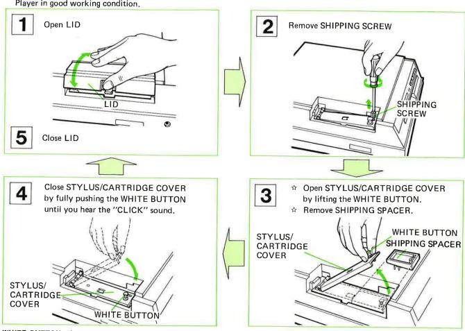
WHITE BUTTON—If the WHITE BUTTON is accidentally pushed while the STYLUS/CARTRIDGE COVER is open, you can't close the COVER. In that case, please lift the BUTTON until you hear the "CLICK" sound, then follow above instruction of "figure 4".
