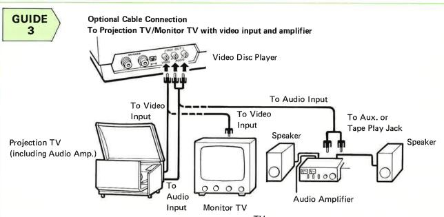
You will need a pin plug type 75 ohm (round) video cable and an audio cables. Neither of these cables is supplied with your Video Disc Player.
