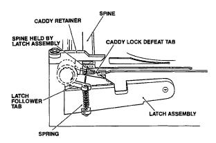
Fig. 1-7. — Spine And Disc In Lock Position
