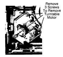
Fig. 2-7. — Turntable Drive Motor Removal
