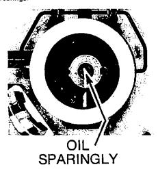
Figure 3-18. Turntable Shaft Bearings
