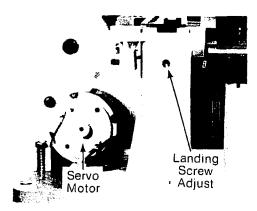
Fig. 3-1. Landing Screw Adjust
