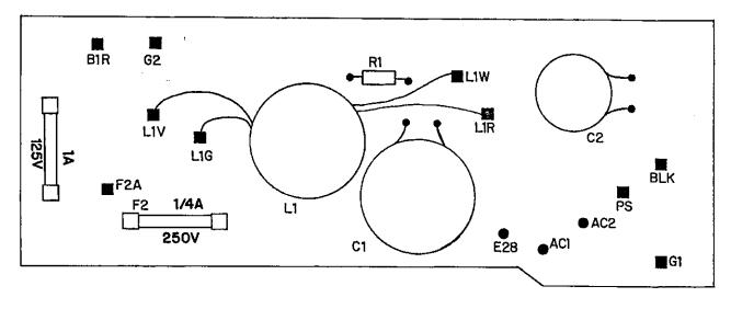
Fig. 5-8. — PW AC IN Circuit Board Assembly
