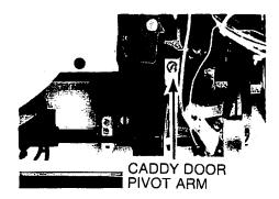
Fig. 3-3. Caddy Door Actuating Pivot Arm
