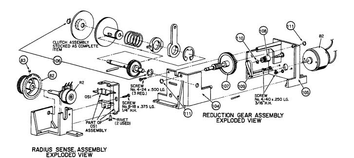
Fig. 2-11. — Radius Sensor And Reduction Gear Assembly Exploded View
