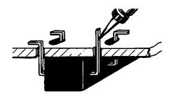
Use Soldering Iron Tip To Pry Leads
