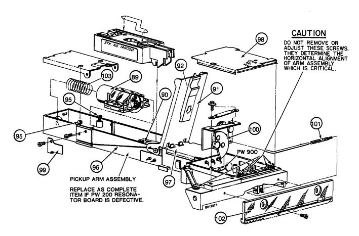
Fig. 2-12. — Pick-up Assembly Exploded View
