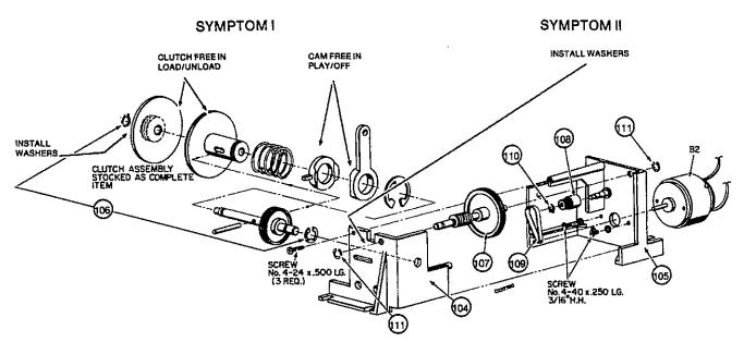
Reduction Gear Assembly Exploded View
