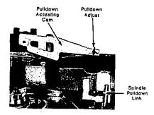
Fig. 3-12. Spindle Pulldown Link
