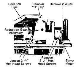
Fig. 2-8. — Reduction Gear Assembly Removal
