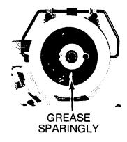
Fig. 3-15. Turntable Lift Slider Cam
