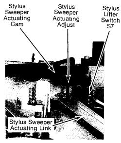
Fig. 3-10. Sweeper Actuating Cam
