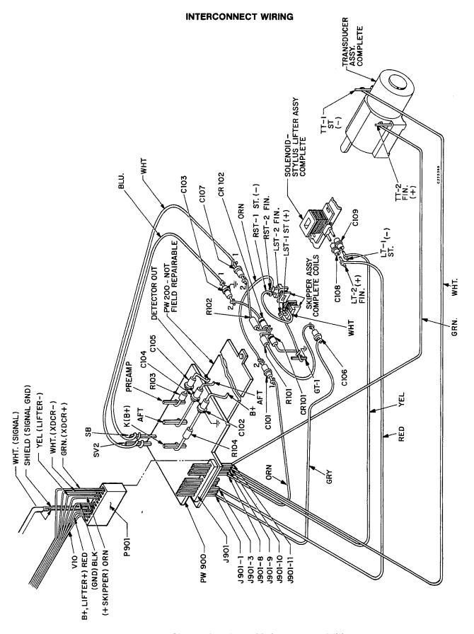
Fig. 5-9. — Pick-up Arm Assembly Interconnect Wiring
