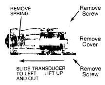
Fig. 2-5. — Transducer Removal
