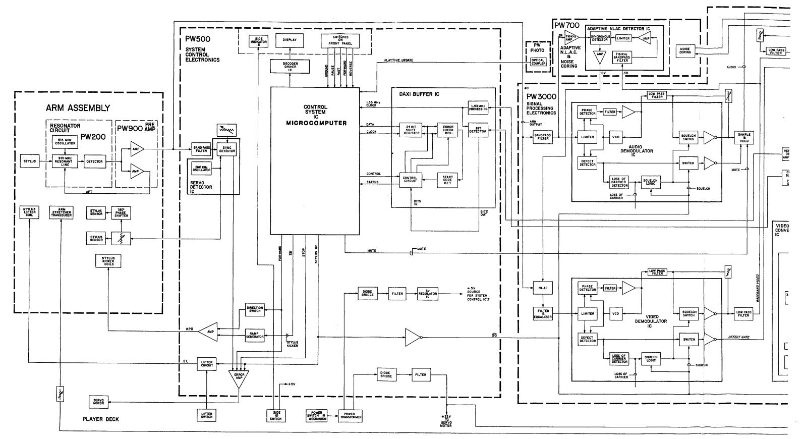
Fig. 1-4. — System Control And Signal Processing Block Diagram
