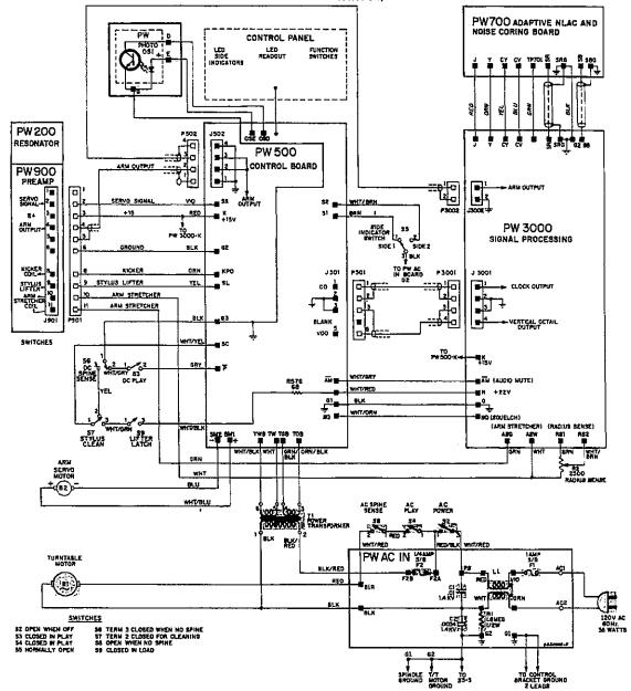
Fig. 1-3. — Overall System Wiring Diagram
