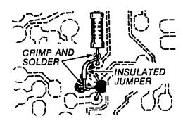
Insulated Jumper Installed
