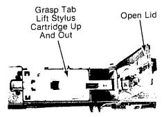
Fig. 2-1. — Stylus Removal Access
