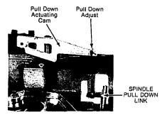
Fig. 3-12. Spindle Pulldown Link
