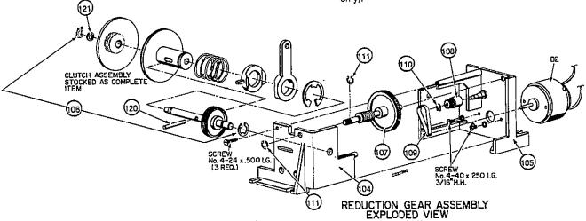
Fig. 2-9. — Reduction Gear Assembly Exploded View
