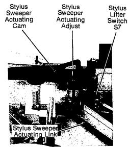
Fig. 3-10. Sweeper Actuating Cam
