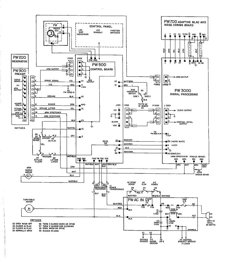
Fig. 5-2. — SFT 100 Interconnect Wiring Diagram
