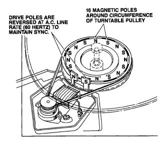
Fig. 1-8. — Turntable Drive Operation
