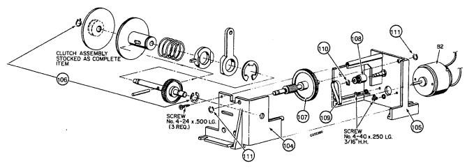
Fig. 2-9. — Reduction Gear Assembly Exploded View
