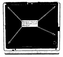
Fig. 2-3. — Bottom Cover Removal
