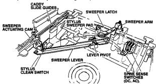
Fig. 1-10. — Sweeper Operation
