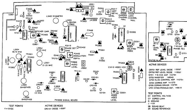
K +15VDC ASI ARMSTRETCHER SET-UP TP3101 ARM INPUT TP3201 COMPOSITE VIDEO BASEBAND TP3202 5.25 MHZ VGO TP3203 FM INPUT
