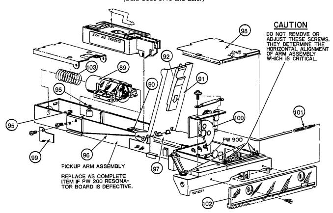
Fig. 2-12. — Pick-up Assembly Exploded View
