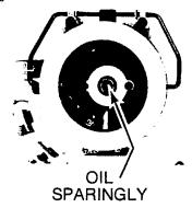
Figure 3-18. Turntable Shaft Bearings
