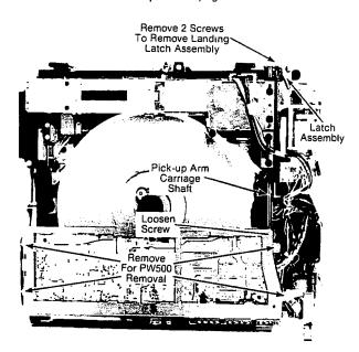
Fig. 2-4. — Pick-up Arm Assembly Removal
