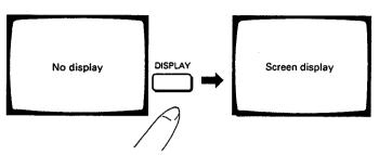
Information regarding the operations being carried out can be displayed on the screen of the monitor TV. When DISPLAY is pressed the first time, the screen display appears.
