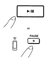
The sound and/or video image disappears and the II indicator lights in the display window. Press ►/II or PAUSE II again to resume playback from the position where pause mode was entered.
