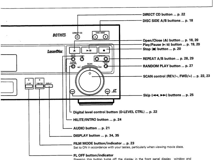
Pressing this button turns off the display in the front panel display window and causes the FL OFF indicator to light. Press the button again to cause the display to return. Turning off the display prevents low levels of noise from adversely affecting sound quality.
