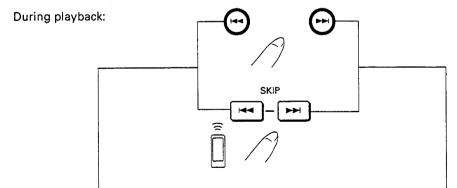
Press once to return the playback position to the beginning of the chaper/track being played. If the button is pressed more than once before the picture reappears, the beginning of a chapter/track located before the chapter/track being played is searched for and played. The position of the located track corresponds to the number of times the button is pressed.
