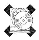
Be Sure to place the disc in the groove on the disc table.
