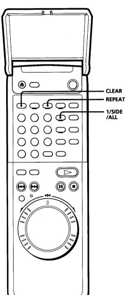
Repeat play allows you to play the disc over and over. You can replay both sides, a single side or one chapter of an LD, and a whole disc or a single track on a CD, or a portion you specified on the disc.
