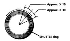
You can also scan a disc by holding down the ◀◀ or ▶► SCAN button on the player while playing the disc. The scanning speed is constant at 10 times the normal speed.
