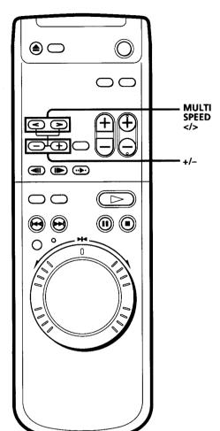
You can find a scene by playing a disc forward or in reverse at varying speeds. There are two ways: using the MULTI SPEED </> and +/buttons, or using the JOG/SHUTTLE ring.
