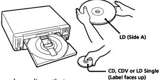
Place only one disc on the tray, carefully fitting it in the circle on the tray.
