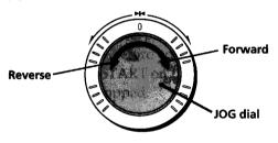
When rotating the SHUTTLE ring: The direction and speed of playback corresponds to the degree you rotate the SHUTTLE ring. The illustration below shows you the approximate positions of each speed (positions are the same for both directions).
