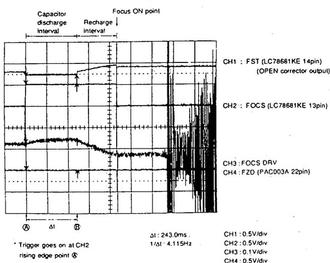
Fig. 5-1-3 FOCS Timing Chart When Disc is Present
