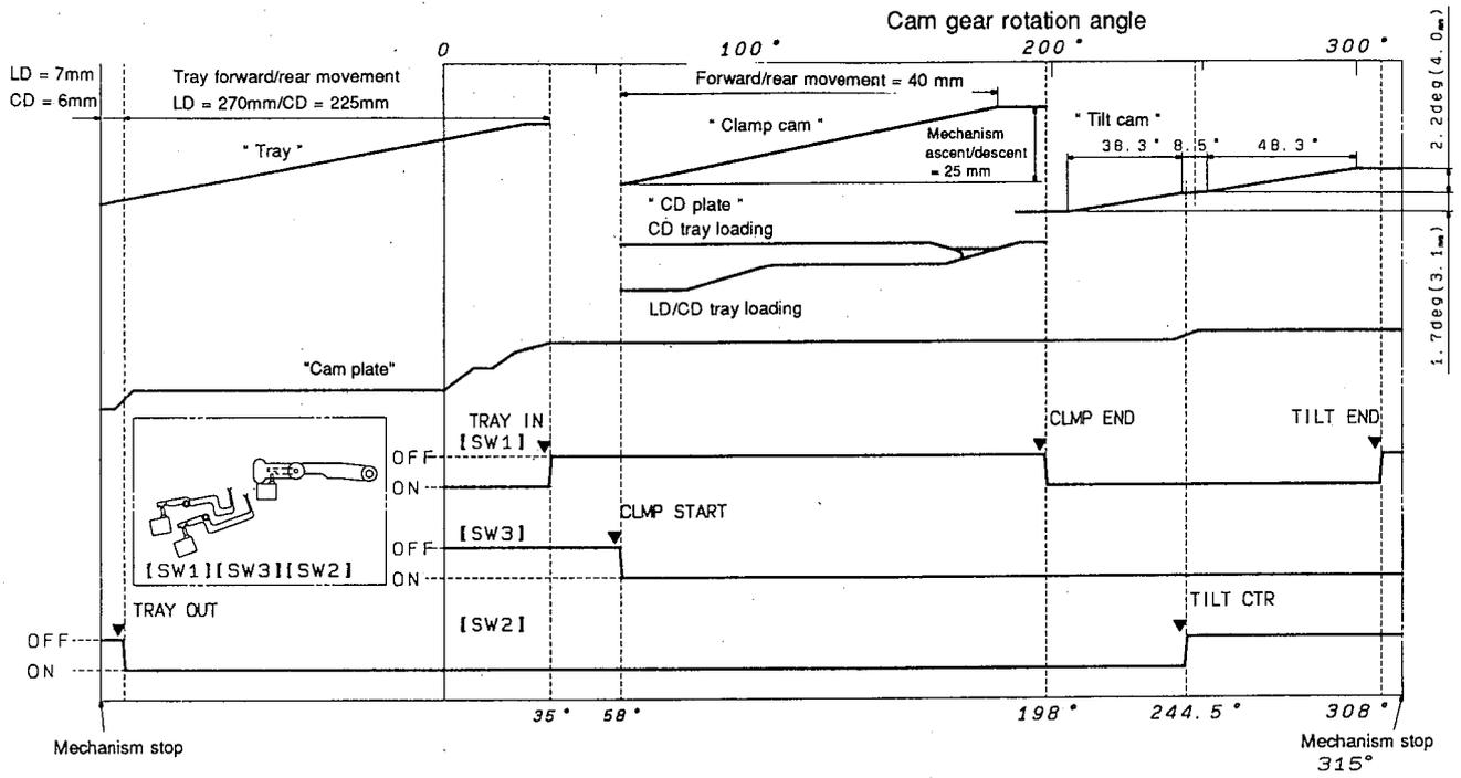
Fig. 2-12 Cam gear rotation angle and position detection
