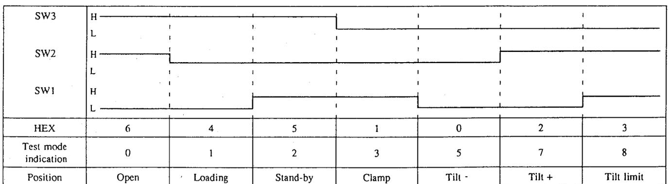
Fig. 4-4-3 Loading/Tilt Position
