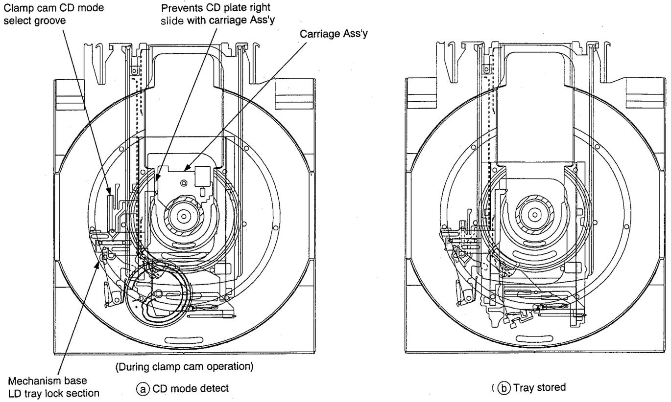
Fig. 2-14 CD Tray open — close operation summary diagram
