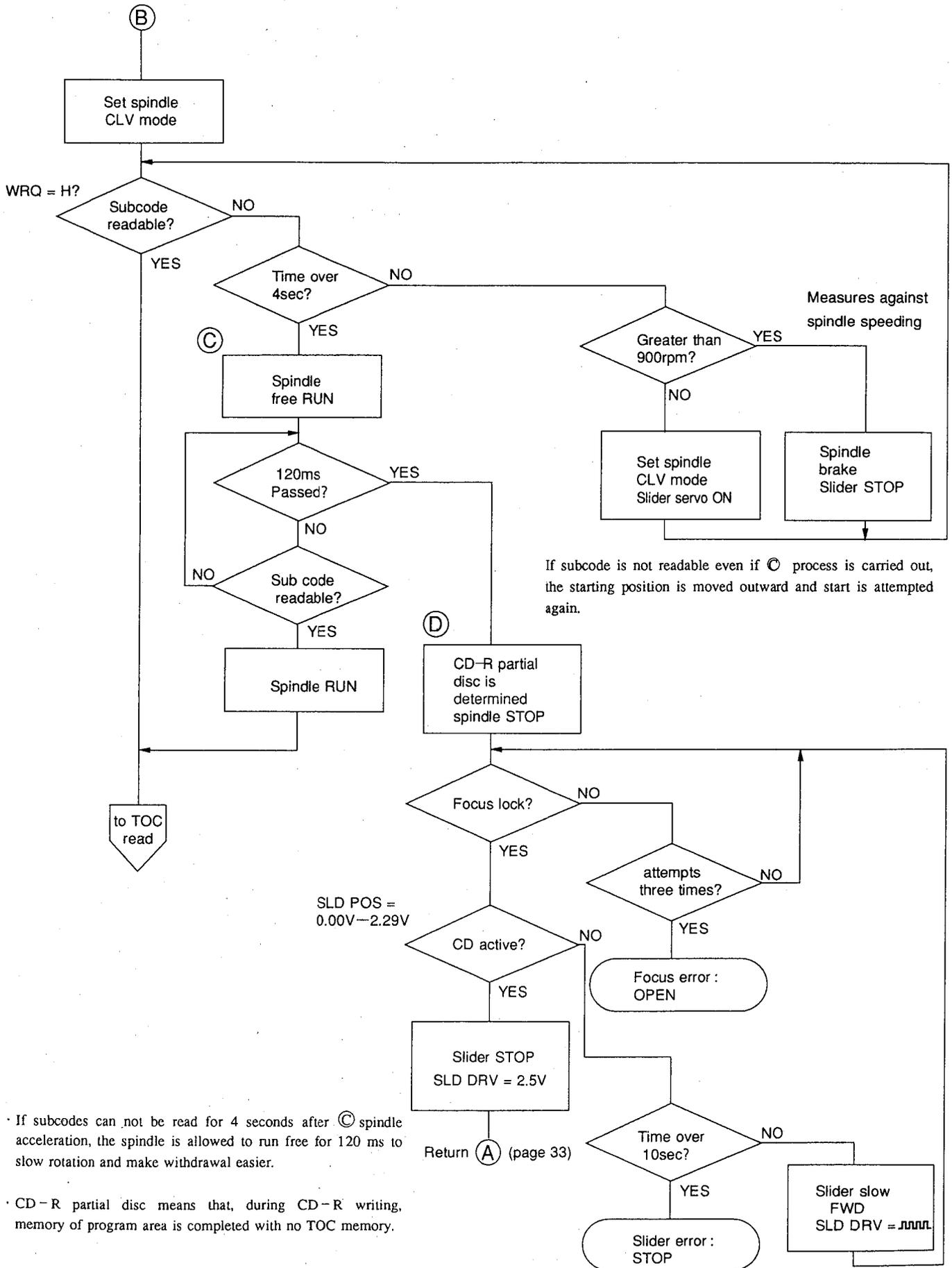
• If subcodes can not be read for 4 seconds after (C) spindle acceleration, the spindle is allowed to run free for 120 ms to slow rotation and make withdrawal easier.
