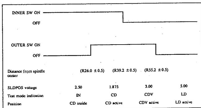
Fig. 4-4-5 Slider Position
