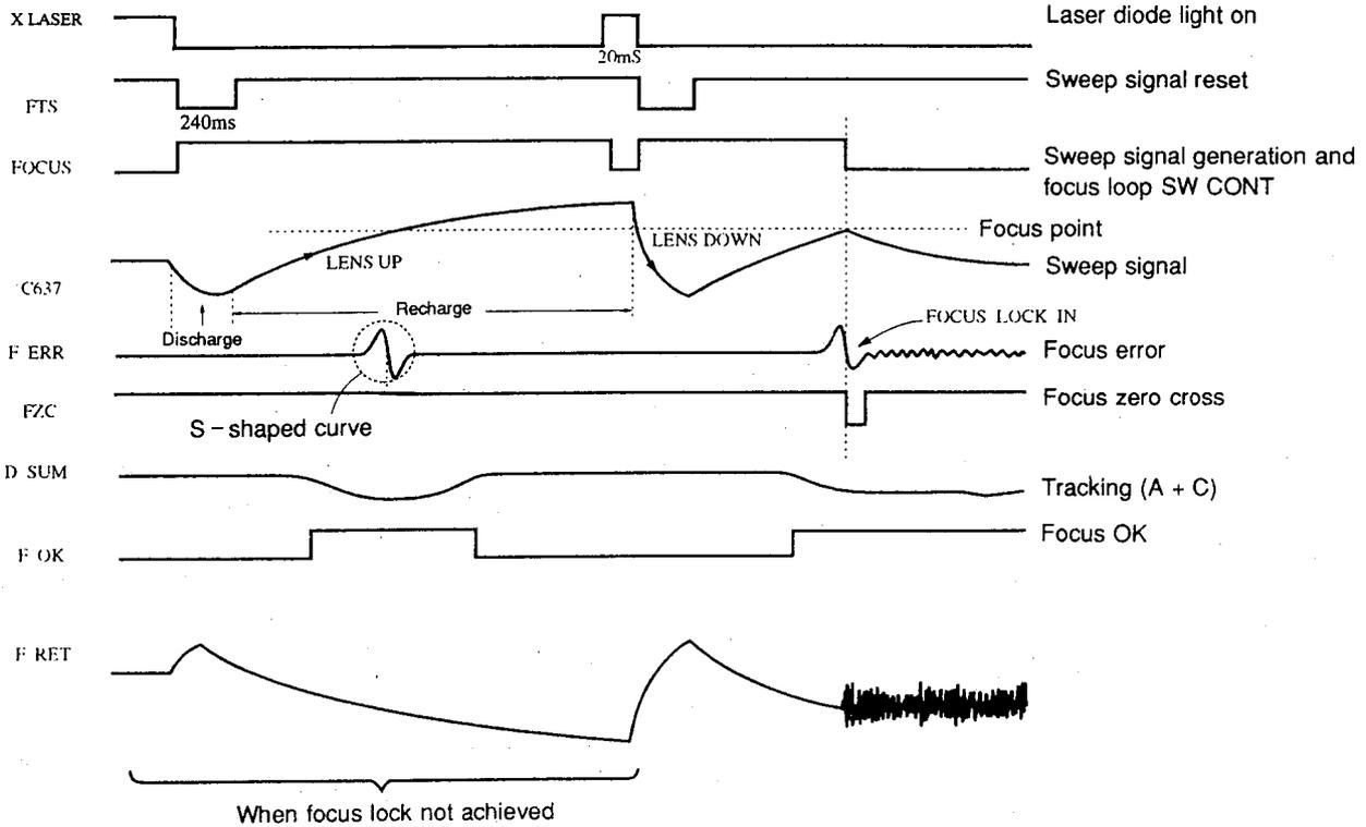
Fig. 5-1-6. FOCS SERVO TIMING CHART
