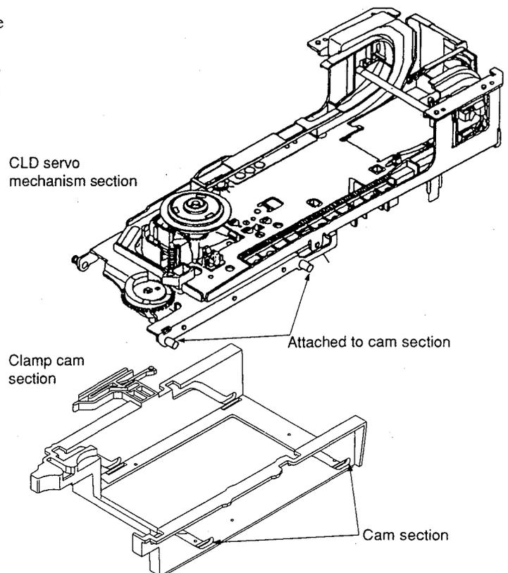
Fig. 2-11 Construction of CLD servo mechanism & Clamp cam section
