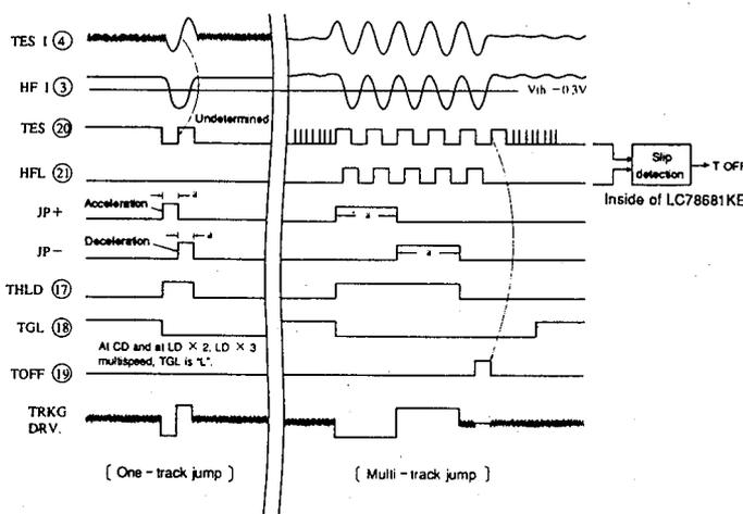
Fig. 5-2-1 Timing Chart for Each Pin Output Signal
