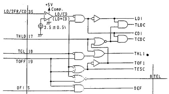
Fig. 5-2-3 TRKG EQ Control Logic Circuit Diagram
