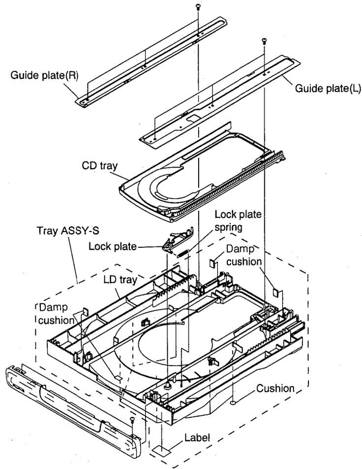
Fig. 2-2 Structure of Tray unit
