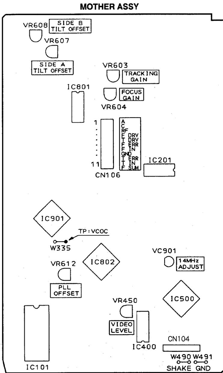
Fig. 20 Adjustment diagram of MOTHER assy
