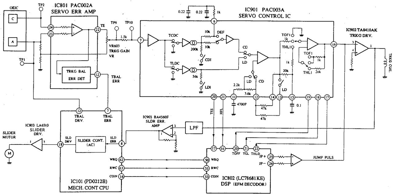
Fig. 5-2-4 TRKG and SLDR SERVO BLOCK DIAGRAM
