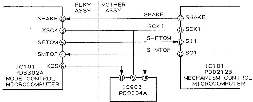
Fig. 4-2 Serial interface connection
