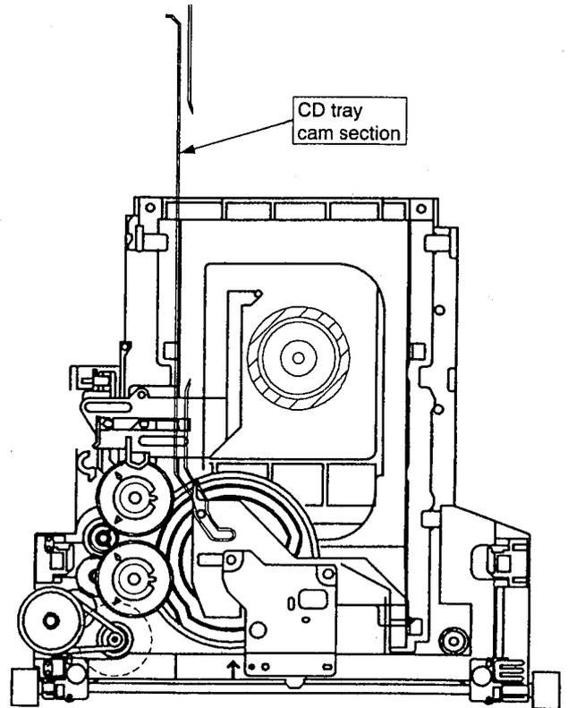
Fig. 2-9 Operation from Tray close to disc clamp & from disc unclamp to tray open
