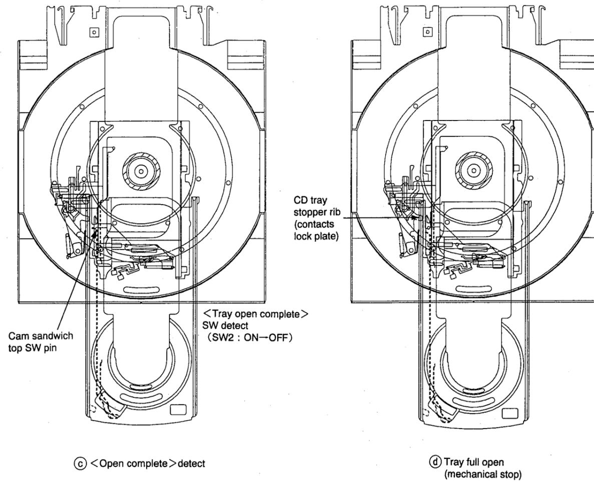
Fig. 2-14 CD Tray open - close operation summary diagram
