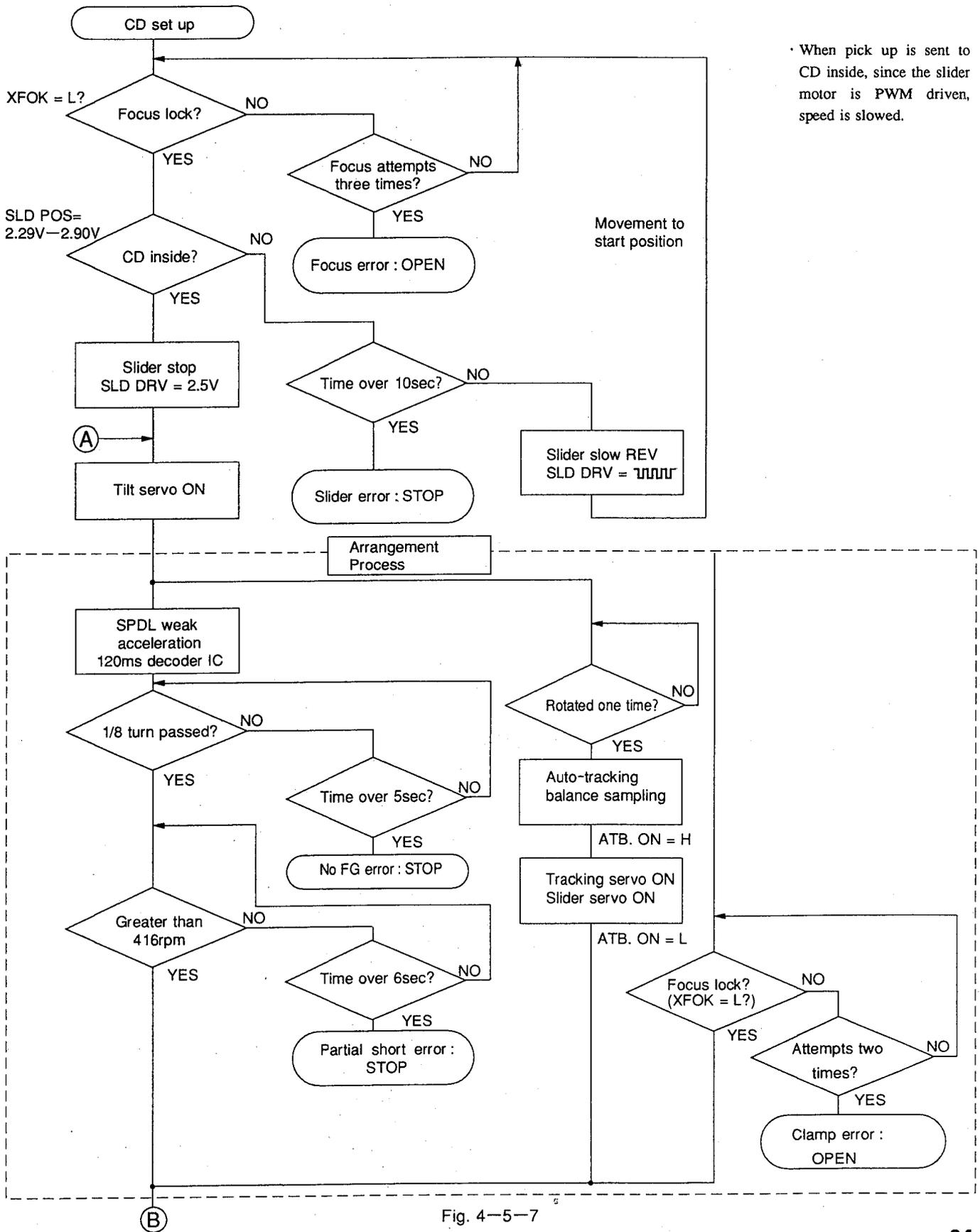
When pick up is sent to CD inside, since the slider motor is PWM driven, speed is slowed.
