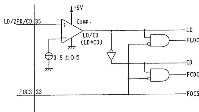
Fig. 5-1-2 FEQ. (FOCS EQUALIZER) Control Logic Circuit Diagram
