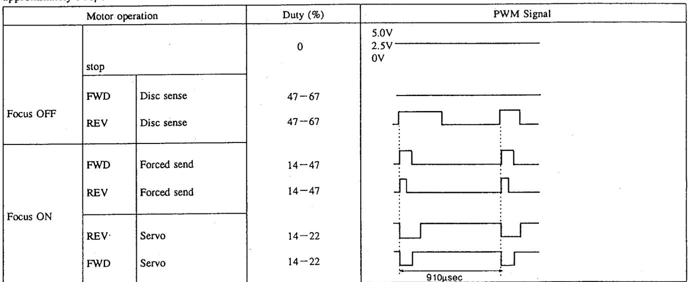
Fig. 4-4-4 Switching of Voltage Impressed on Slider Motor
