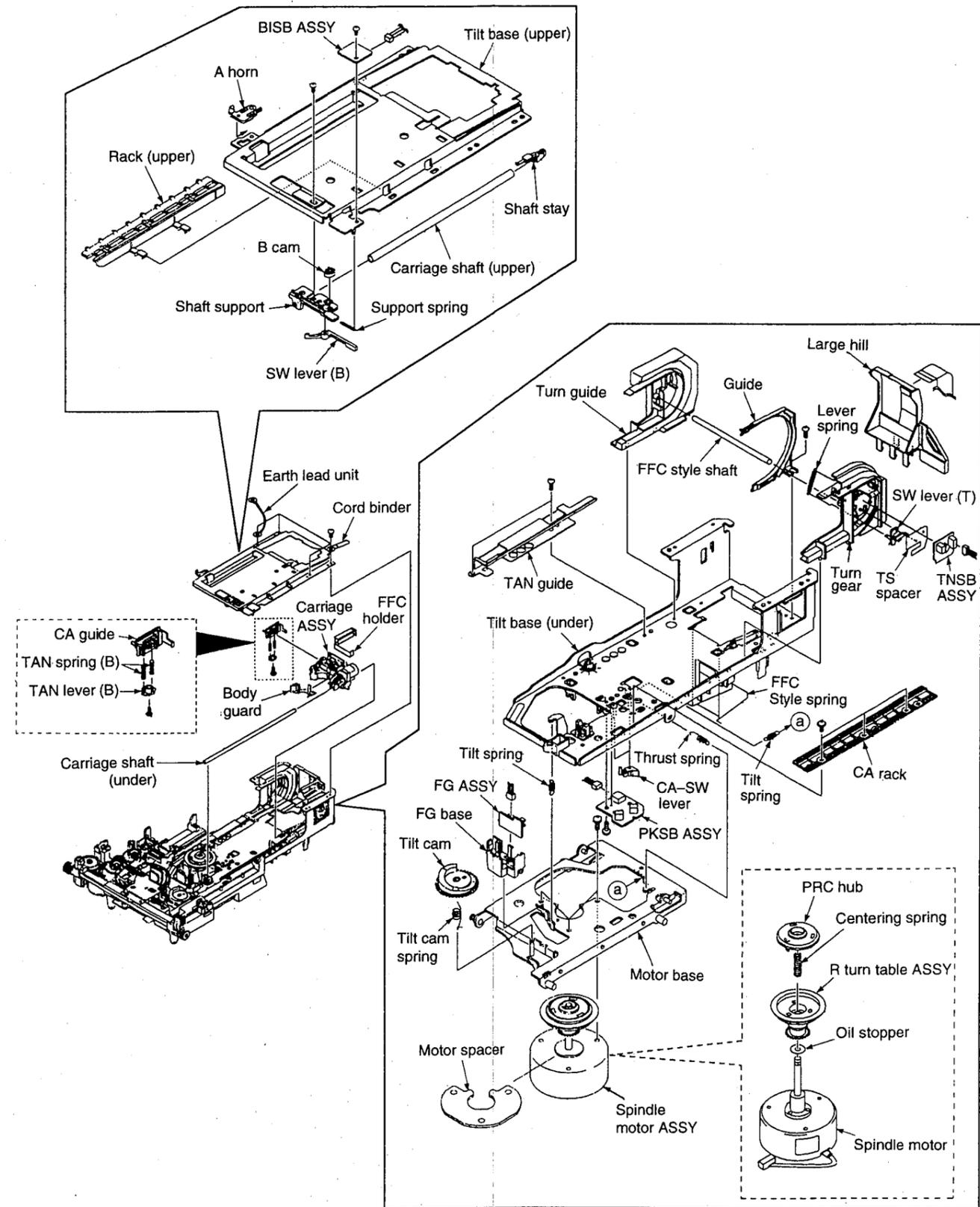
Fig. 2-15 Servo mechanism section disassembly diagram
