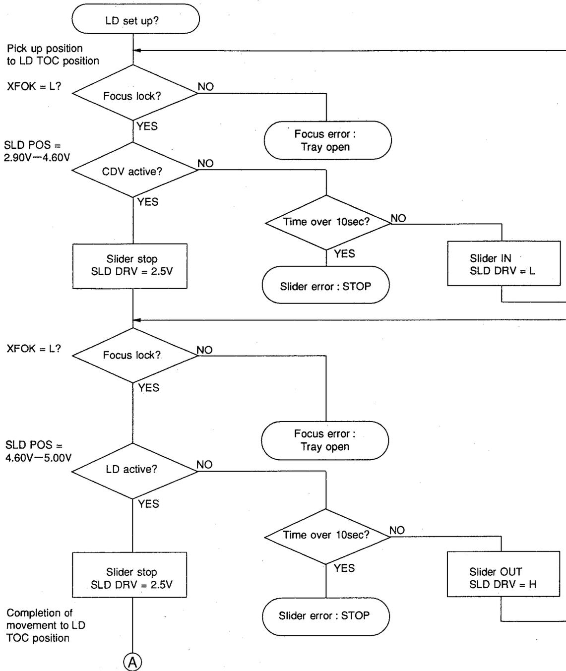
During movement to spindle start position, if the focus is cannot be achieved, it is determined that there are overlapping LD, CD and the tray is opened.
